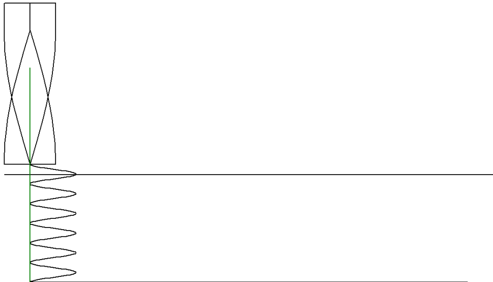
The Helical Plunge Move Example of Pitch
