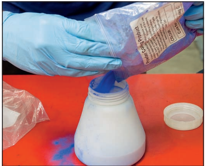
7 Pour the powder into the spray cup. There needs to be at least an inch in the bottom for the gun to work, but it doesn't matter if you fill the cup and don't use it all, as you can save it and reuse it again.
