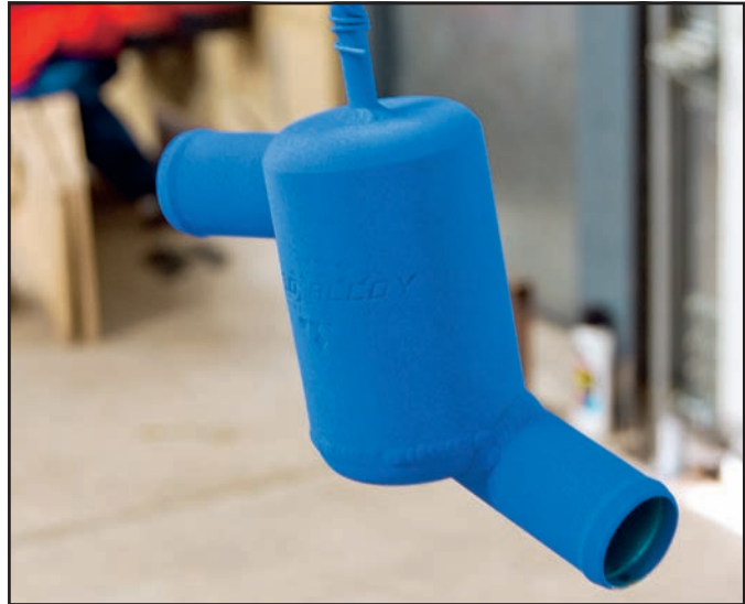
12 The coated item will have a very textured and dull finish. Have a look to ensure it's completely covered. If not, coat areas which need it.
