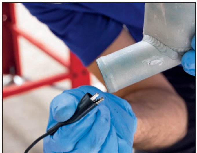
10 With the part thoroughly de-greased and securely hung in position you can connect the earth lead from the powdercoating machine.
