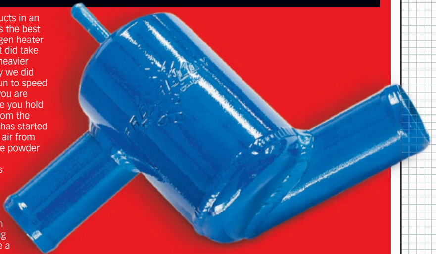
14 Time to cure the powder, we used a halogen heater. When the powder starts to gloss over it is at the correct temp to cure. Leave for around 10mins. Allow the product to cool slowly before handling.
