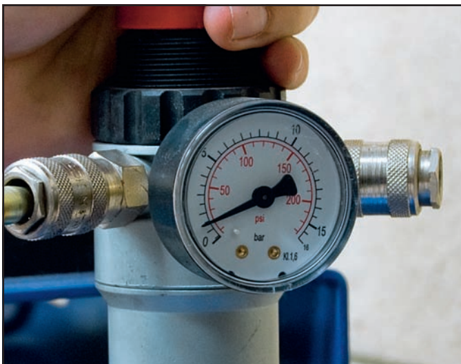
4 The compressed air only needs to be between 10 and 15psi to ensure a constant spray. The air gun can take up to a feed of 150psi, but can be regulated by the screw in the base of the gun handle.
