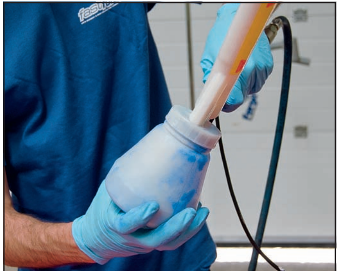
8 Screw the cup onto the gun, ensuring that the power supply to the kit is still OFF at this point.
