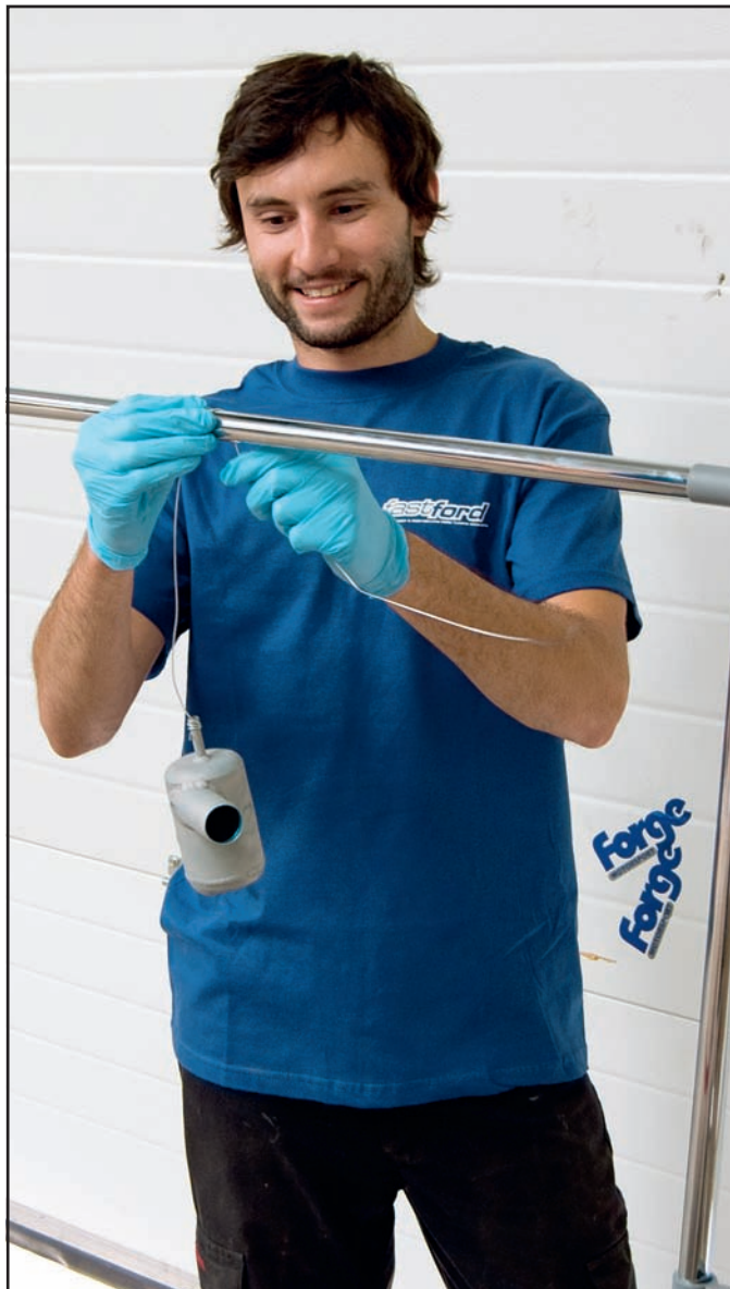
6 Hang the product ready for powdercoating. We used a cheap clothes rail, which was ideal because it was easily adjustable and gave great access to the product.
