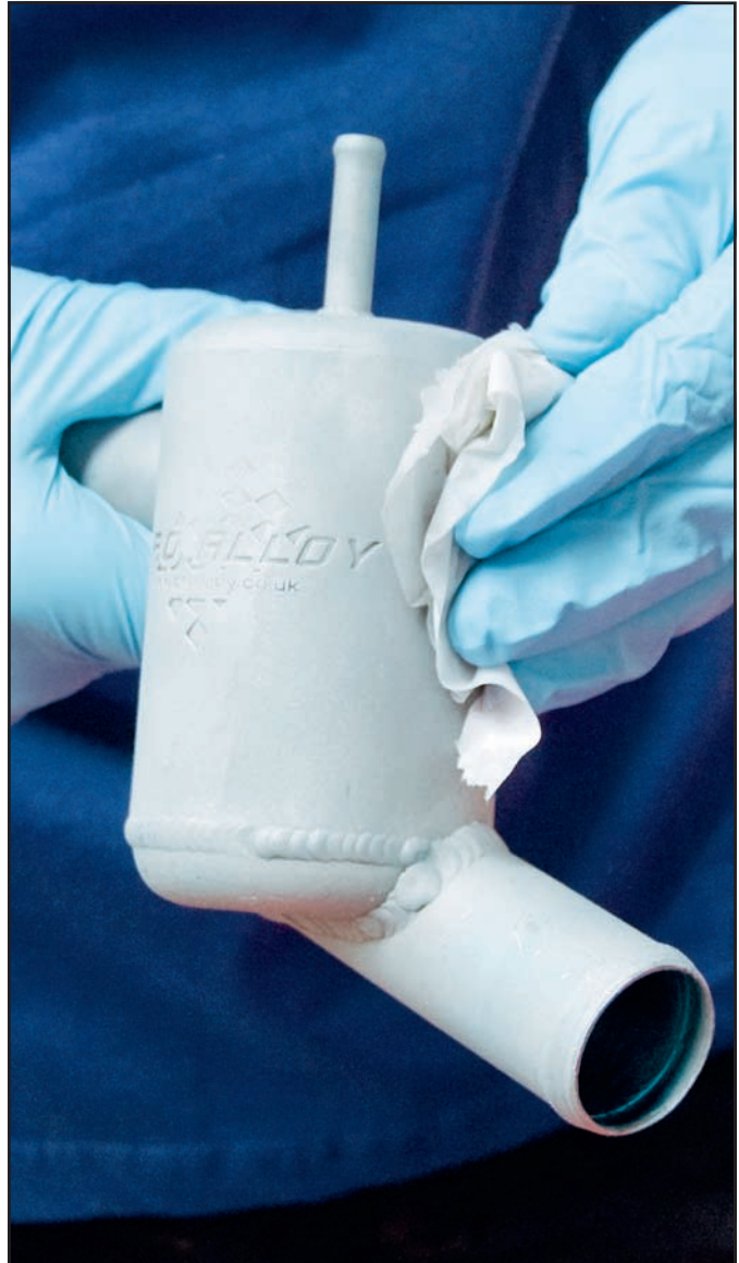
5 Thoroughly de-grease the part to be coated to make sure that the surface is as clean as possible. Use a lint free cloth so fibres don't adhere to the product and leave imperfections under the powdercoat.
