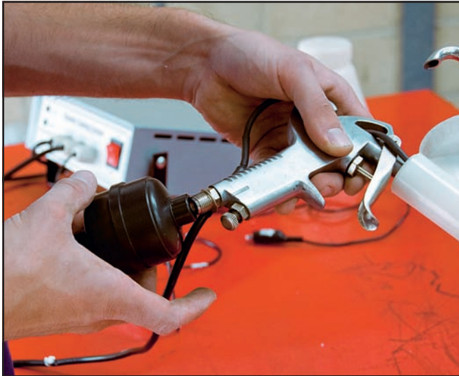
3 Fit the disposable water trap to the bottom of the spray gun. This ensures that no moisture in the compressed air mixes with the powder.
