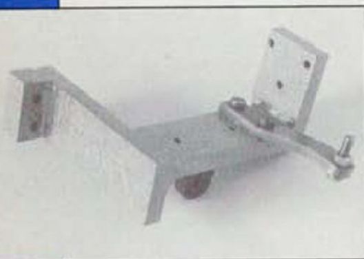
Bracket which supports the motor. Readers will probably need to modify this in detail to suit their particular motor.
