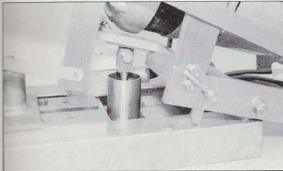
Illustration above shows how the dashpot provides support to the saw on its return stroke. Below, a rear view of the completed saw.
