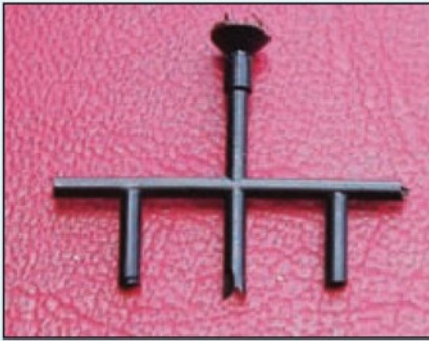
11. Completed moulding of Tee piece.
