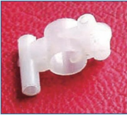
14. Completed gearbox moulding.
