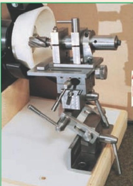
9. Sharpening the end teeth of an end mill with the rest mounted at the side of the wheel and at the right hand end.
