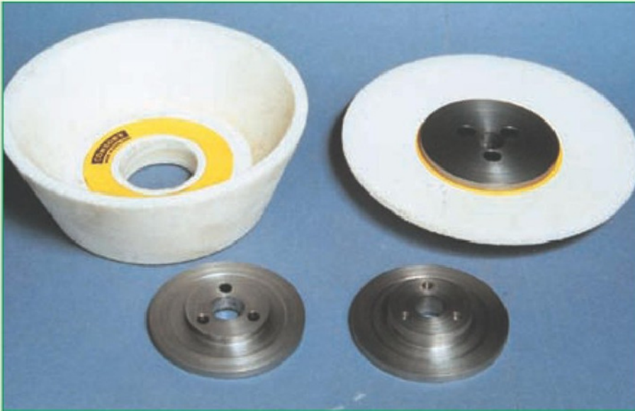
6. The two grinding wheels and the flanges for adapting the large hole in the wheels onto a smaller spindle diameter.
