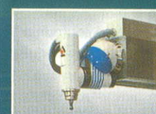
Electrospindle adapted to an Automatic Head, 4,5 to 21kW, 20.000 to 30.000rpm
