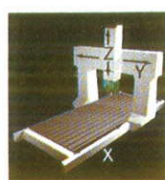
Three linear axes (X, Y, Z) are driven with the FZ 35 machine in principle.
