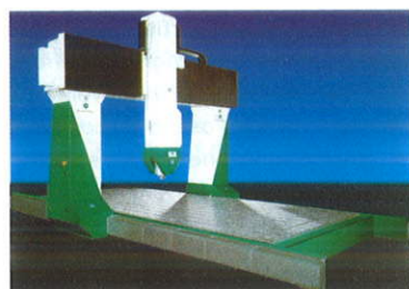
Three linear axes (X, Y, Z) are driven with the FZ 35 machine in principle.
